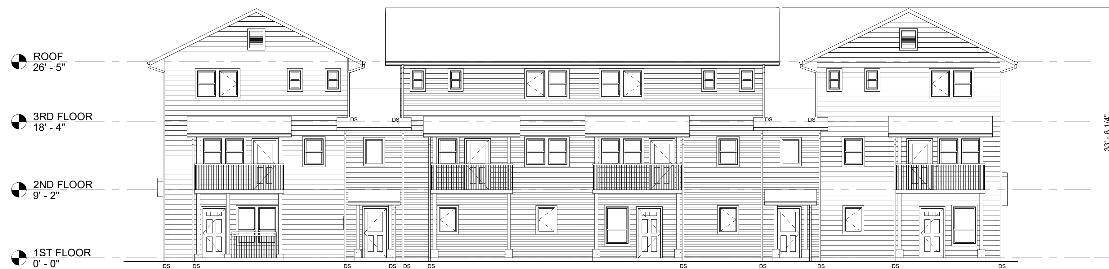
1 BUILDING ELEVATION - FRONT A5 1/8" = 1'-0"
