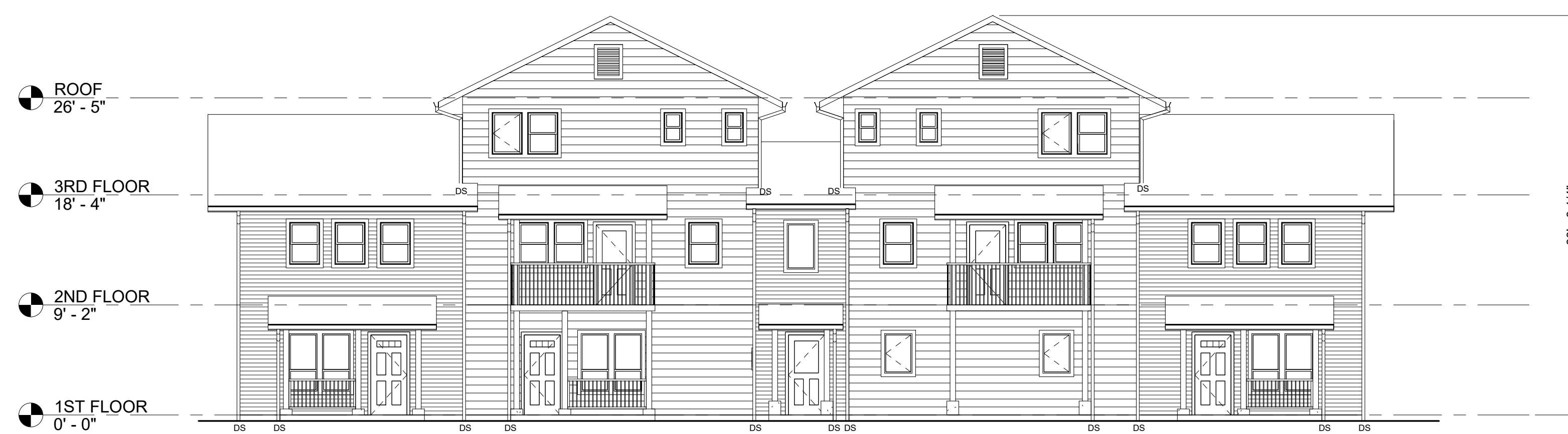
1 BUILDING ELEVATION - FRONT A3 1/8" = 1'-0"
