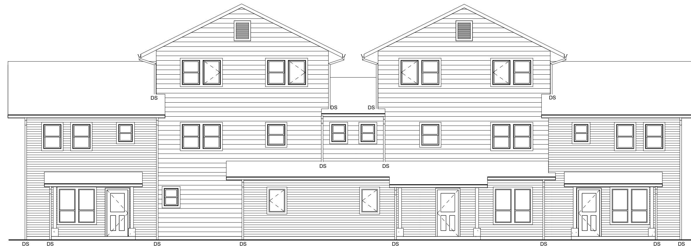
4 BUILDING ELEVATION - BACK A3 1/8" = 1'-0"
